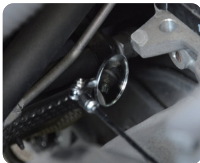
38 mm Diameter Inspection Mirror
